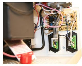
2. Press firmly on connectors to secure them to the Propane Burner Controller. Secure the Buck Boost Converter plugs by screwing in the set screws, previously loosened.
