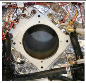
2. Install a new mounting gasket into place.
