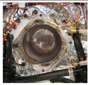
1. Clean the boiler tank's front plate.
