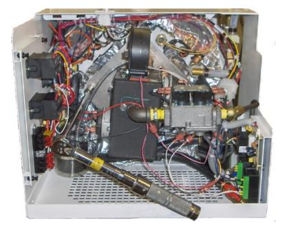
3. Using a 9/16 socket wrench with a wobble extension, tighten the three nuts securely.
