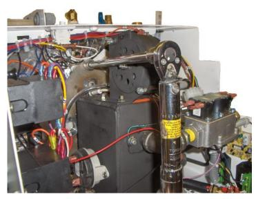
1. The Propane-Burner is secured to the Aqua-Hot with four nuts that can be removed by using a 9/16 inch socket wrench with a wobble extension.
