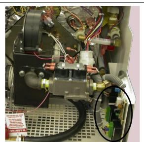
Locate both the Propane-Burner's white, electrical plug connection to the Propane-Burner Controller and both of the green plug connections to the Buck Boosts.
