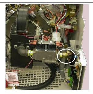
1. Locate the gas valve assembly on the Propane-Burner and the corresponding fuel lines.
