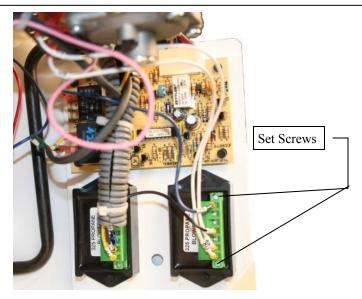
2. Loosen the set screws, securing the green plugs to the buck boosts,
