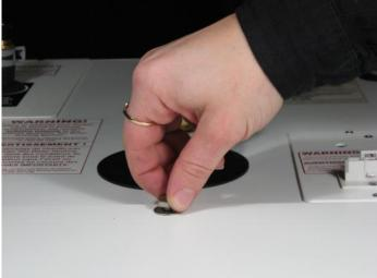
3. Unscrew the bolt securing the top of the cover in place. Figure 39
