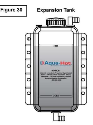
The antifreeze and water heating solution should be filled to the "HOT" level on the Expansion Tank when the Aqua-Hot is at the maximum operating temperature.
