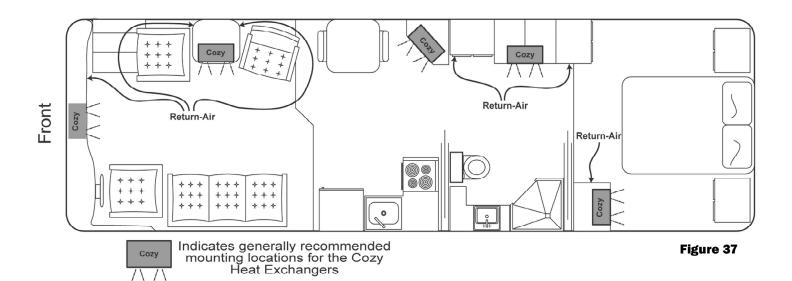
**NOTE:** This is just a sample for mounting locations of the Cozy heat exchangers. Actual placement and quantity may vary on the individual design of the RV. For questions or assistance, contact Aqua-Hot at +1 (800) 685-4298.
