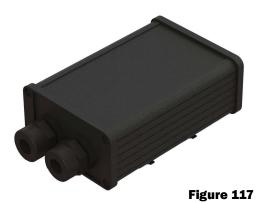
The diesel burner controller operates all the components of the diesel burner head and safely shuts the heater OFF in the event of an overheat, flame-out, and low voltage condition. It also receives diesel burner operation status signals from the flame sensor, control thermostat/ETS Module, and DC high-limit thermostat.
