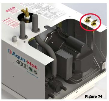
Using a  $^7/_{16}$ " wrench, loosen the nuts securing each fuel line to the Aqua-Hot.
