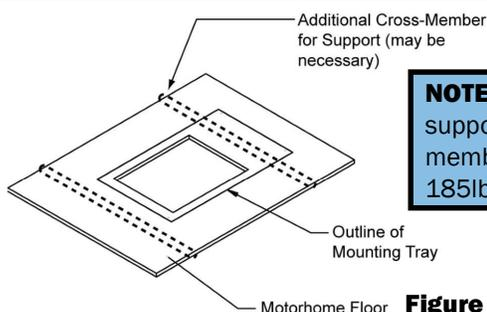
**NOTE:** The Aqua-Hot must be supported by structural cross-members that can support at least 185lbs.
