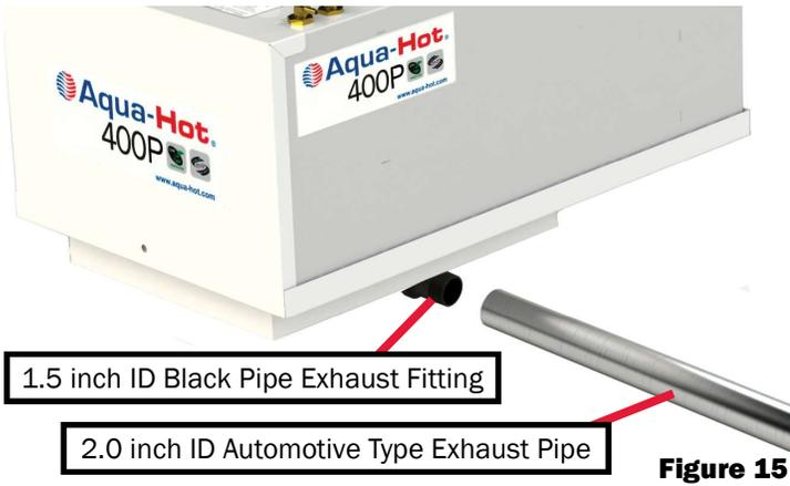
**NOTE:** A maximum of three 90° bends are allowed in the exhaust pipe. Also, the exhaust pipe cannot be longer than 27.5 feet.
