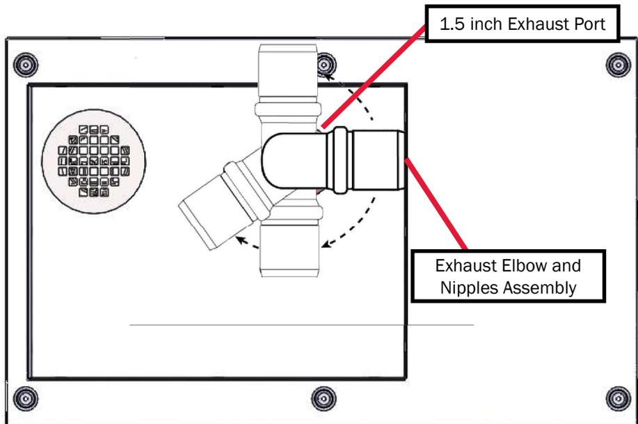
**NOTE:** The exhaust elbow can be rotated 270°, as shown in the illustration; however, the exhaust must not terminate beneath the vehicle or beneath an open-able window or vent.
