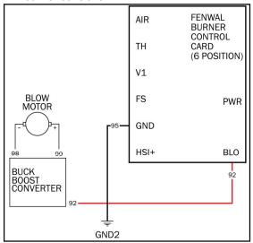
4. Verify that the Propane Burner Controller is sending a ground signal to the buck boost converter at the GND pin, on the Controller.
