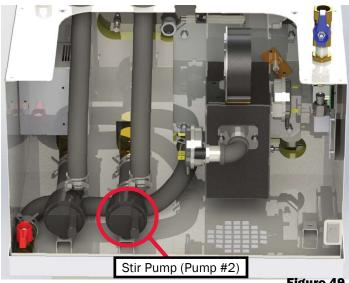
Troubleshoot the stir pump if there is a lack of hot water or the Reporter is showing an OVER-CURRENT fault for the pump.
