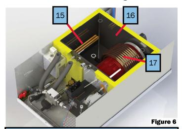
**NOTE:** The top panel has been made transparent in the view above to aid in the explanation of the heater. DO NOT remove the top panel. Doing so risks irreparable damage to the Aqua-Hot. Only remove the service panels.
