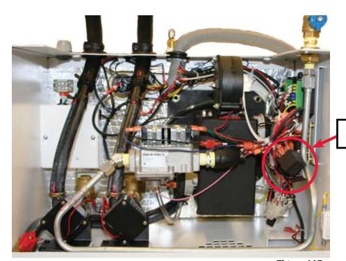
Fan Validation Switch Relay
