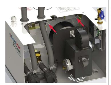
Finger tighten all four nuts previously removed to secure the propane burner to the boiler tank.
